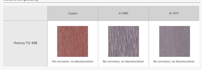
Total Immersion Corrosion Test (ASTM F 483)
