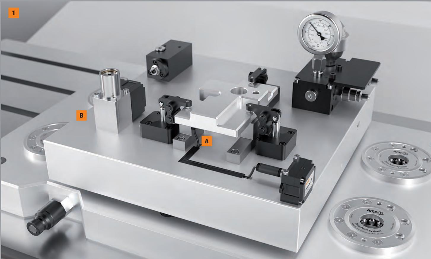
The hydraulic clamping fixture is provided with two queries. The workpiece location pad is queried via a microswitch **A** with a connected Sender-Unit. The wireless pressure switch **B** monitors the pressure of the clamping fixture hydraulic clamping circuit.
