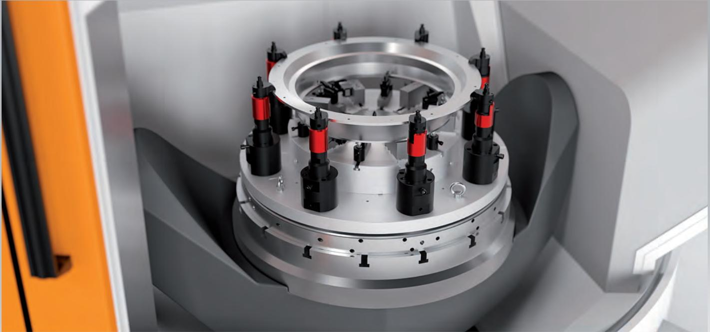
In the milling and turning process, cables are often in the way due to the changing positioning of the rotary table or do not offer the necessary flexibility in order to follow the movements of the fixture. By using the AMF Wireless sensing systems, the workpiece support can be queried easily and with process reliability and without laboriously laying cables.
